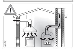
▶ Great care should be taken when using the cooker hood at the same time and in the same room or area of the house as another heating appliance which depends on the air in the room. Such appliances include gas, oil, wood or coal-fired boilers and heaters, continuous flow or other water heaters, gas hobs, cookers or ovens which draw air in from the room and duct exhaust gases out through a chimney or extraction ducting.
